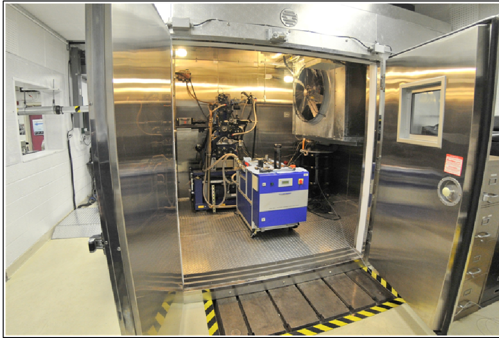
Fig. 3.5. Optically accessible engine enclosed in the environmental chamber
